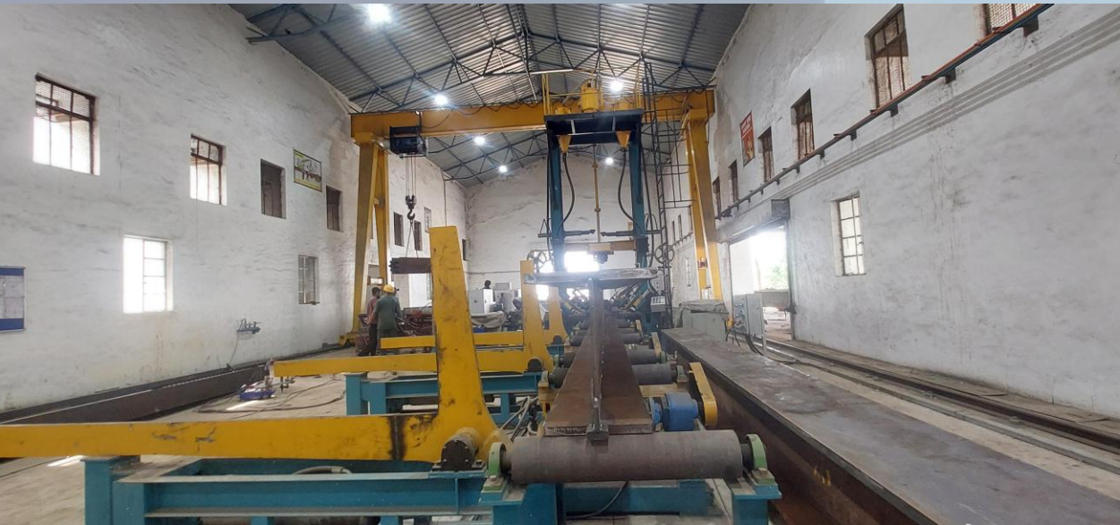
Girder Fit Up on Vertical Beam Welding M/C
