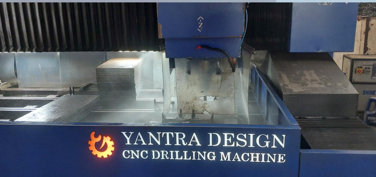
CNC Drilling (Splice/Gusset Plates)
